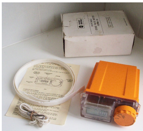
Illustration 1: PDRM82 Modifying/Fixing a Plessey PDRM 82
